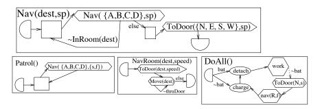
Figure 3: The remainder of the PHAMs for the Deliver–Patrol domain. *Nav(dest,sp)* leaves route choices to be learned through experience. Similarly, *Patrol()* does not specify the sequence of locations to check.
