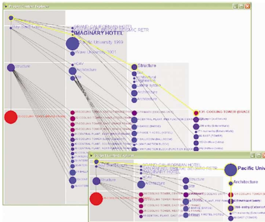
Figure 11 Screenshots of the CoMem Project Context Explorer. The window is resizable. Each object is positioned in the vertical axis according to its level of granularity, and in the horizontal axis according to its degree of interest with respect to the focal point.
