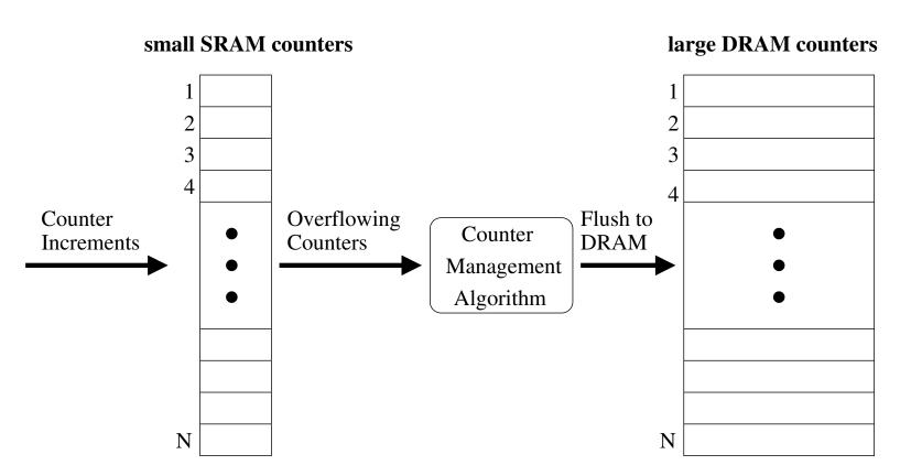
Figure 2: Hybrid SRAM/DRAM counter architecture
