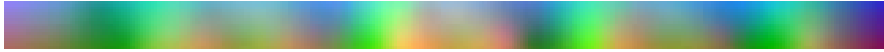
Figure 3: Map of one corridor ( 32.5m by 1.7m ) calculated from 58 sample images. Each sample is projected using each of the first three eigenimages. The resulting three values are assigned to the colors red, green and blue. Points between the samples are obtained by interpolation.
