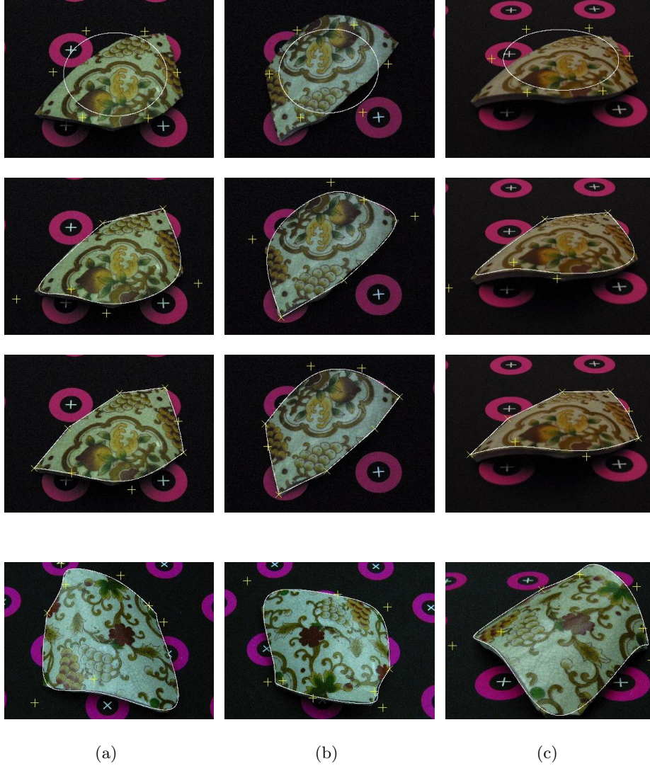
Fig. 4. Results are shown for two pot shards. Projections of the control points are drawn as yellow '+' for untagged and yellow 'x' for tagged ones, and the corresponding subdivision curve is drawn in white. Six views are used for the fitting process of the first shard, while only four are used for the second shard. In both cases, two of those are shown in columns (a) and (b). The third column (c) shows a view that is not used for fitting and is taken from a lower angle than all other images.
