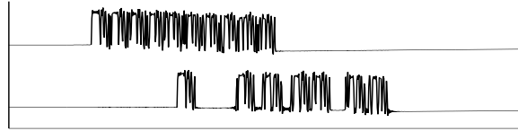
Figure 3: A REF burst (top) is “stretched” as the TEST system is unable to keep up with the continuous burst of data (bottom).
