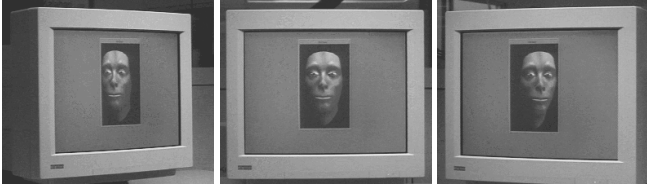
Figure 6. Three frames of a view through a Handicam while DECface tracks a user in 3D using color stereo.
