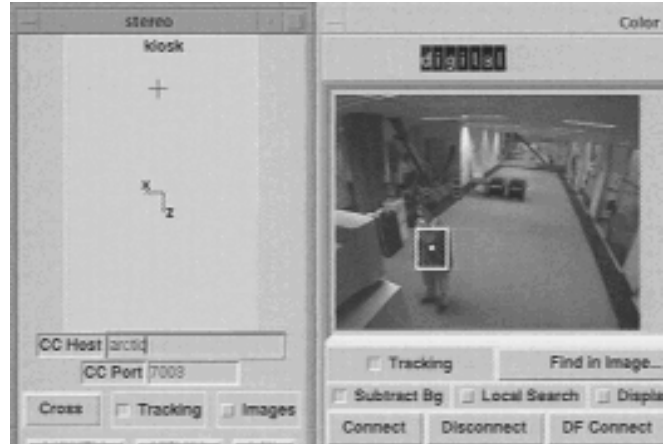
Figure 2. Sample output from the color tracking module. Images were obtained from the right camera of the stereo pair. The left hand portion of the display shows a plan view of the scene with a cross marking the 3D location of the individual projected onto the ground plane.
