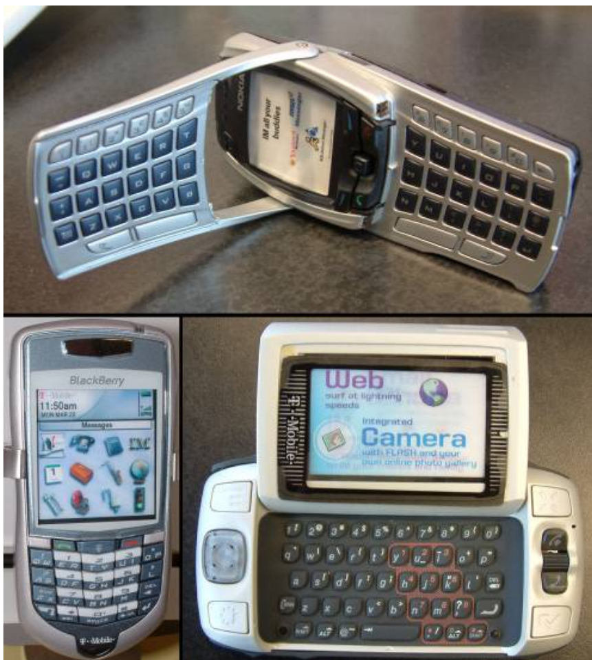
Figure 1: Commercial mobile phones with mini-QWERTY keyboards: Nokia 6820 (top), RIM BlackBerry (bottom left) and Danger/T-Mobile Sidekick (bottom right).
