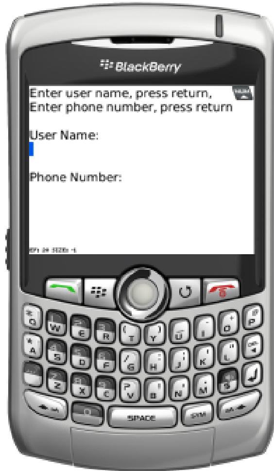
Figure 11: The mini-QWERTY keyboard enabled mobile phone used in the mobile study: the RIM Blackberry Curve 8320.
