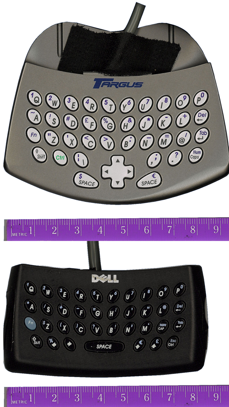
Figure 2: The mini-QWERTY keyboards used in both studies: Targus (top) and Dell (bottom) keyboards. Keyboards shown in the figure are actual size.
