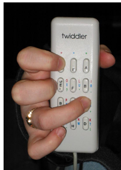
Figure 1. Chord for the letter 'j' (R0L0) on the Twiddler
