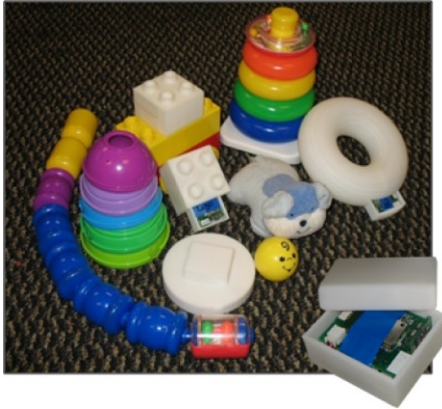
Figure 5: Commercial Toys with augmented counterparts in white. The sensor units exposed to show how they are embedded
