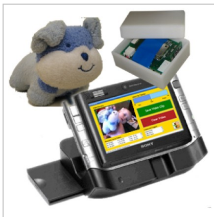
Figure 1: Child'sPlay components consist of sensor augmented toys and a mobile computing platform to receive data
