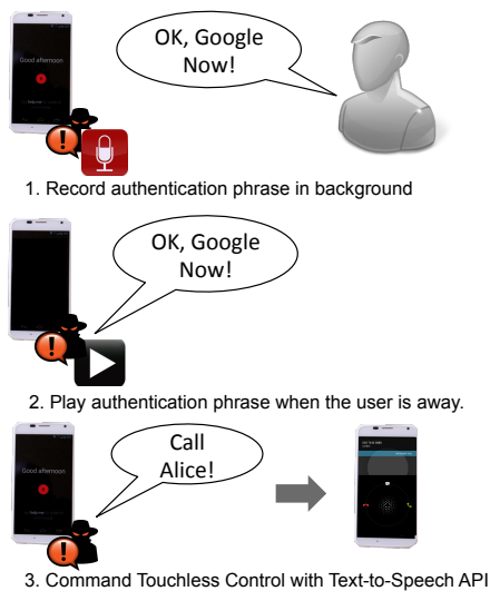
Figure 9: Workflow of the attack on the Moto X's Touchless Control. Malware in the background can record a user's voice, and replay it to bypass voice authentication.
