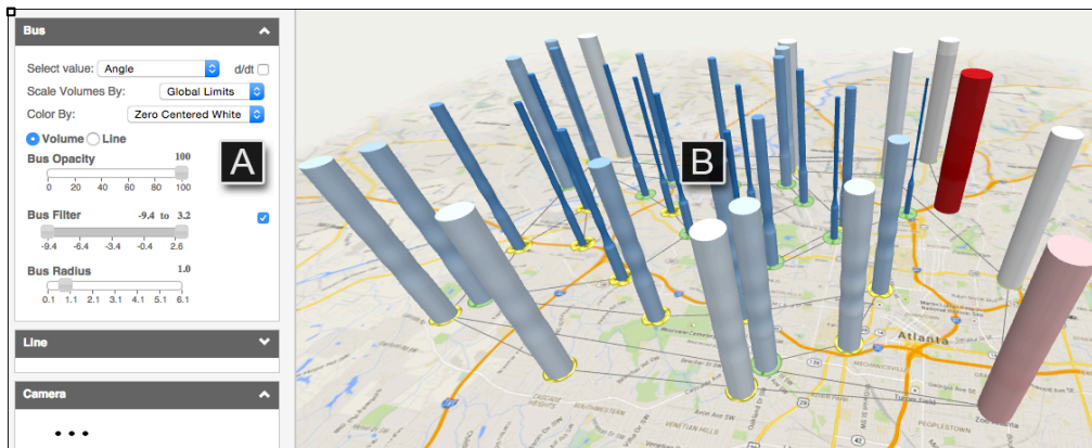
Figure 2: STEPS's main view is composed of (A) the control panel and (B) the 3D network view. Here the 3D network view illustrates the changes of a desired variable, through time, for each bus. The control panel allows users to select the visualized attributes, visual bus and line characteristics (such as opacity or height), filter out values, adjust the cameras, and many other features.
