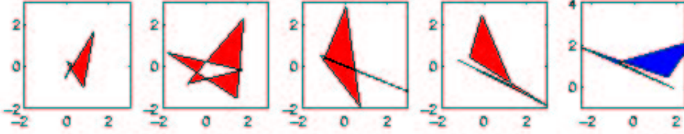
Figure 1: Given a set of range estimates with no odometry, these are the intermediate steps of the Levenberg Marquardt algorithm in determining 2D coordinates for all robots. The resulting configuration is an inverted transformation of the true values (last frame).
