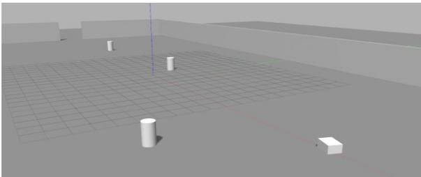
Figure 2: Gazebo simulation environment. The cylinders represent pedestrians, and the box represent the robot.
