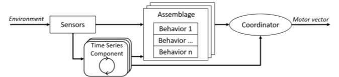
Figure 6: In a traditional behavior-based architecture, sensor measurements feed directly into the relevant behaviors. Here, the TBATS model is treated as another percept in parallel with other sensor measurements.
