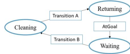
Figure 5: FSA for janitor robot
