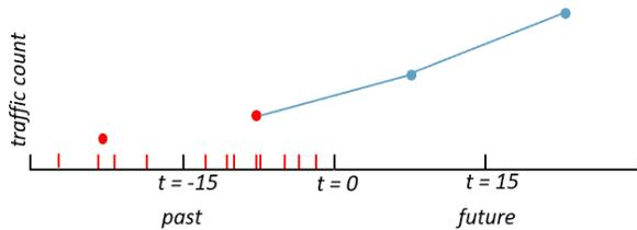
Figure 4: Predicting traffic counts at any time based on past values (red) and forecasted future values (blue). Red dashes are individual detections; red circles are the final count per period
