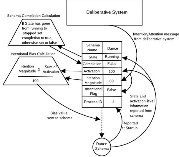
**Fig. 7** Dataflow in the intentional bus. Arrows show origin and destination of the data. Trapezoids show computations internal to the intentional bus.
