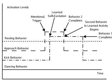
**Fig. 12** An idealized graph of activation values for a learned routine soccer behavior. In this example, after the approach behavior becomes active, the kick behavior's activation increases via self-excitation in anticipation of being active next.
