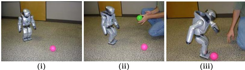
**Fig. 19** Depiction of high intention soccer plan. i) QRIO approaches the ball ii) The operator tries to distract QRIO with the green ball (the releasing mechanism for the greet behavior) iii) QRIO kicks the ball and completes the plan.
