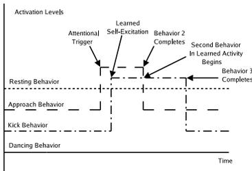
**Fig. 12** An idealized graph of activation values for a learned routine soccer behavior. In this example, after the approach behavior becomes active, the kick behavior's activation increases via self-excitation in anticipation of being active next.
