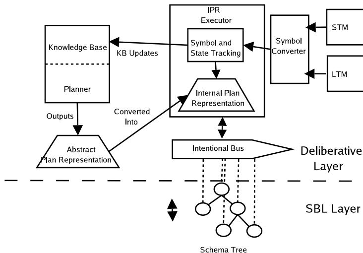
**Fig. 14** Overview of the end-to-end deliberative/reactive architecture
