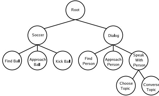
**Fig. 4** Example behavioral tree in the EGO architecture containing two main behaviors: Soccer and Dialog
