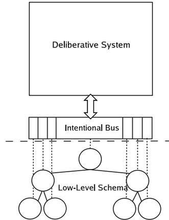
**Fig. 5** Overview of the interaction between the deliberative system, intentional bus, and lower level reactive behavior
