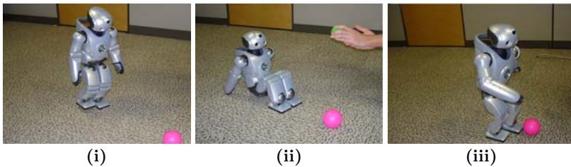
**Fig. 22** Depiction of low intention soccer plan. i) QRIO approaches the ball ii) The operator tries to distract QRIO with the green ball, the lower intentional bias of this plan allows the greeting behavior to run and QRIO greets the user and sits down. iii) QRIO gets back up, continues executing the plan, and kicks the ball.
