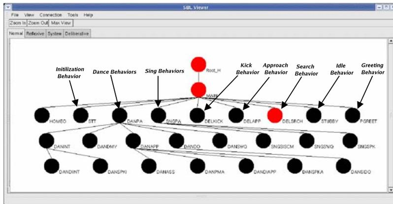
**Fig. 15** Behavioral tree used in intentional experiments. The bold-italic labels indicate the behavior associated with that node and any of the node's children if applicable.
