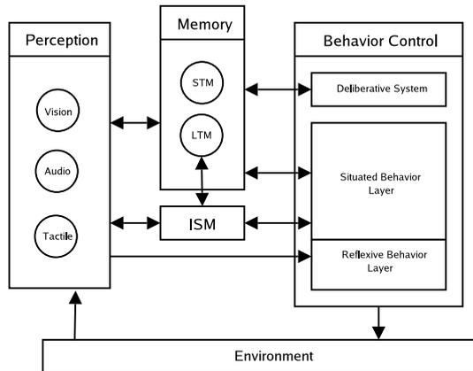
**Fig. 3** Overview of the EGO architecture. Short-term memory and Long-term memory are denoted by STM and LTM respectively.
