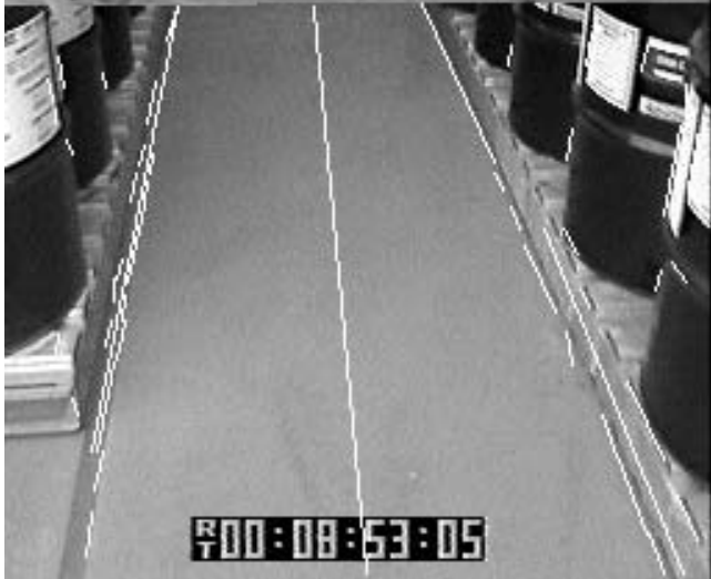
Figure 3. Example of an accurate FLF centerline determination.
