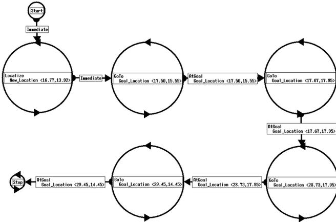
Figure 4: FSA for the path shown on Figure 3. The main building blocks in this case are GoTo motor schemas and AtGoal perceptual triggers.
