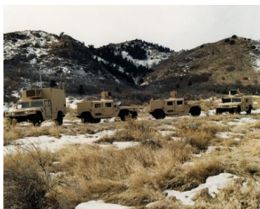
Fig. 1. A team of four robotic scout vehicles manufactured for DARPA's Demo II project. The formation techniques reported in this article were implemented on these robots. Photograph courtesy of Lockheed-Martin.
