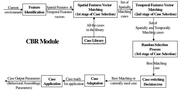
Figure 1. High-level structure of the CBR Module
