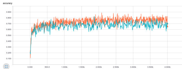
Fig. 2. Training (orange) and validation accuracy (blue) for a fine-tuned Inception network (best seen in color).
