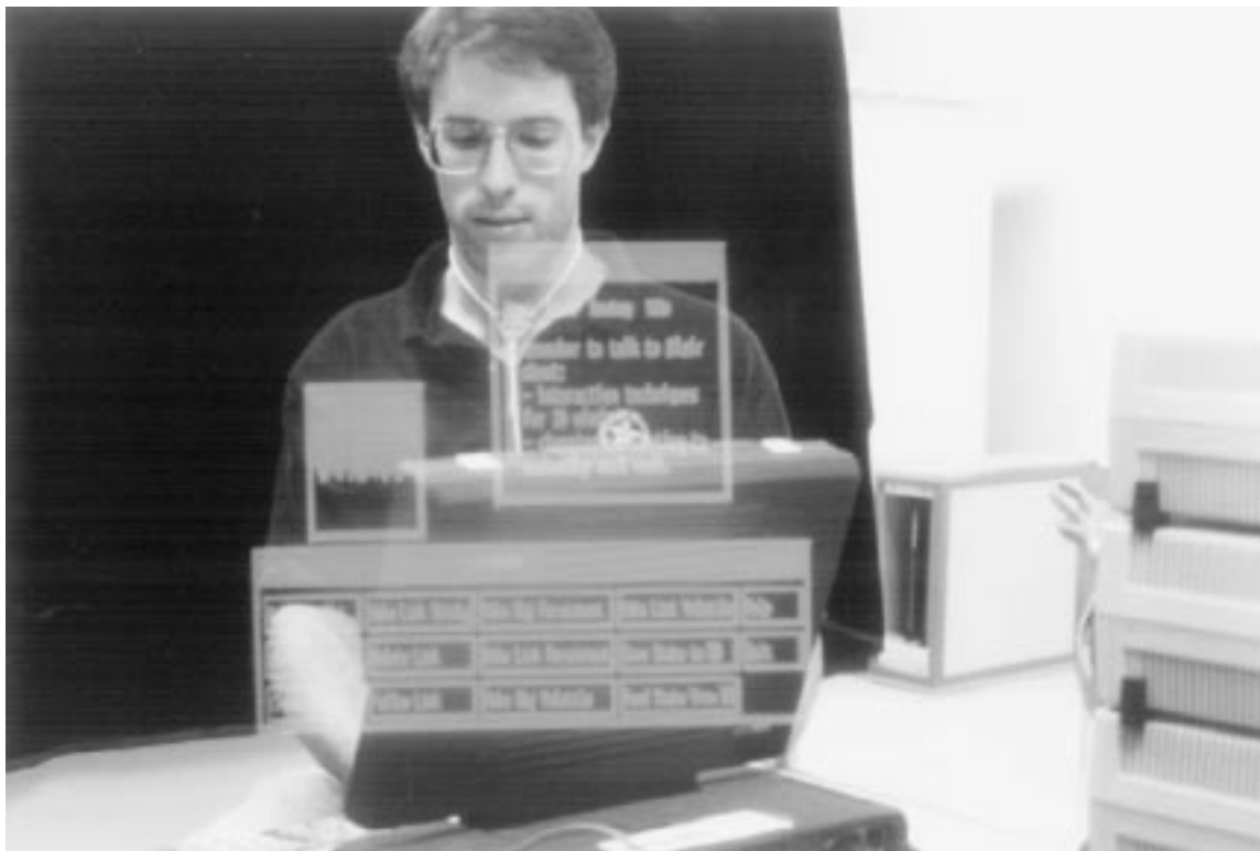
Figure 4: A note is attached to a tracked person and a load-average meter to a 3D location.
