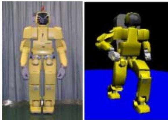
Figure 1: *HRP1 humanoid robot and running simulation*
