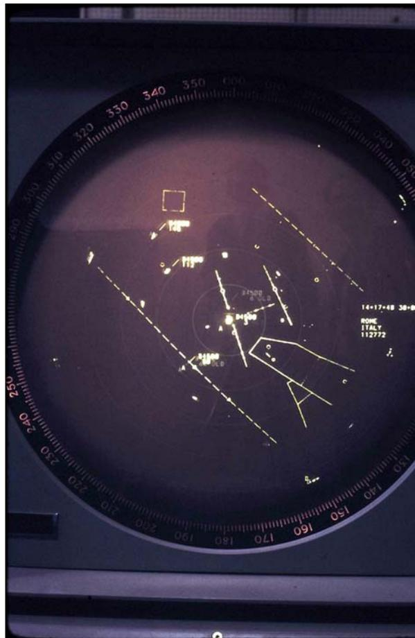
Figure 2 – Air Traffic Control Display mixing raw and computer generated symbols
