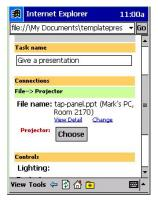
Figure 3: A partially configured template. In this case the user has selected the file to be presented but has not yet selected the projector.
