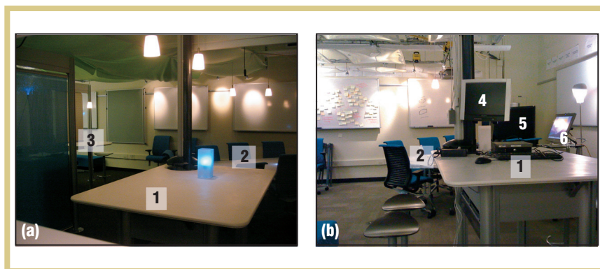
Figure 2. The inSpace environment (a) before and (b) after hardware installation: the (1) arrive space, the (2) assemble space, and the (3) aside space. The hardware installation includes a (4) kiosk display on a swiveling arm in the arrive space, an (5) inSpace Wall display at the head of the inSpace Table, and a (6) movable Podium touch display.
