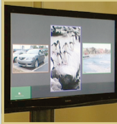
Figure B. An inSpace Wall, displaying artifacts shared by three meeting participants. A meeting participant (green) is uploading a new file to the inSpace Wall, indicated by the status bar on the lower left.
