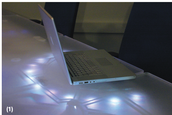
Figure A. Lighting feedback on the inSpace Table. (1) Feedback indicates that the laptop computer is connected to the meeting room. (2) Selected lighting animations used by the inSpace Table. The inSpace Table promotes fluid transitions between personal and shared workspaces.
