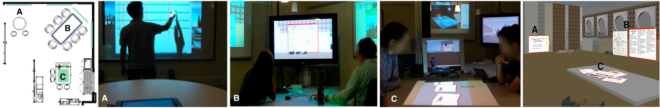
Figure 2. Three collaboration regions in the inSpace team room and the connected virtual space in brainstorm mode. Aside wall (A) centers around a large interactive whiteboard. Assemble/array (B) uses three wall displays configured around a sensing table. Aside table (C) combines an interactive tabletop and vertical display. Remote participants inhabit the virtual space and communicate with co-located collaborators using spatialised audio and telepointers.
