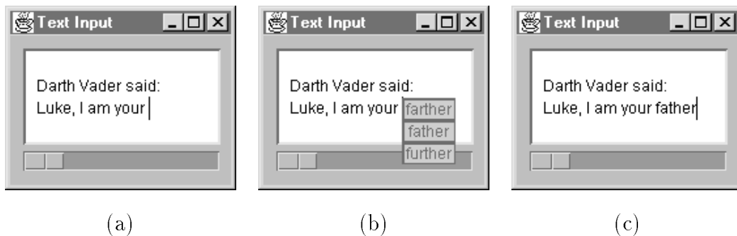
Fig. 9. This is an application that shows text typed by the user. We have hooked a word predictor up to the toolkit and now the application also shows word prediction results. (a) The word predictor before the user types the letter f. (b) A mediator asks the user which word prediction is correct. (c) The result
