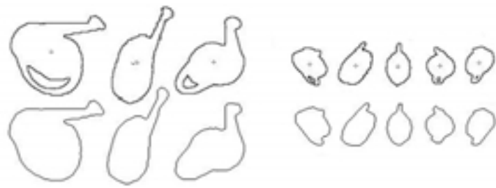
8 Shadow contours (top) and interpolated polygons (bottom) from a watering can (left) and a teapot (right). The current version of our software doesn’t handle holes in the contours yet.
