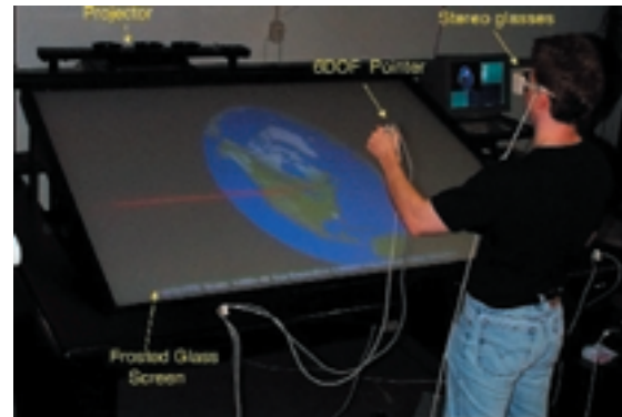
1 A user interacting with Georgia Tech's Virtual Workbench using a 6 degrees-of-freedom (DOF) pointer.
