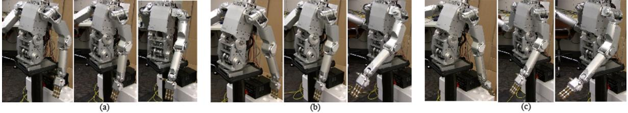
Fig. 3. Tennis swing motion with (a) simulation-in-the-loop, (b) feedforward & feedback, and (c) eigenphysics secondary action techniques.
