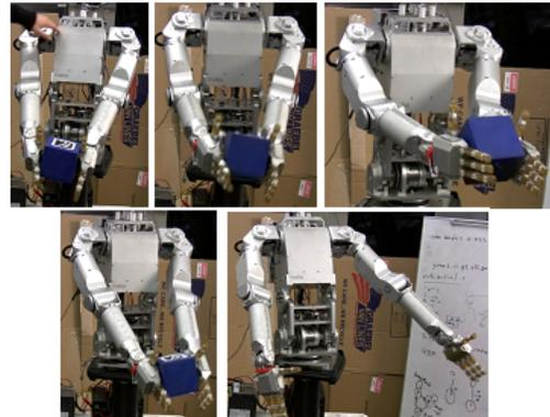
Fig. 6. Pushing the robot during a box-moving trajectory to demonstrate secondary action from external forces using eigenphysics.
