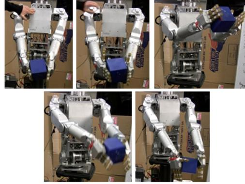
Fig. 5. Pushing the robot during a box-moving trajectory to demonstrate the response using feedforward & feedback for secondary action.
