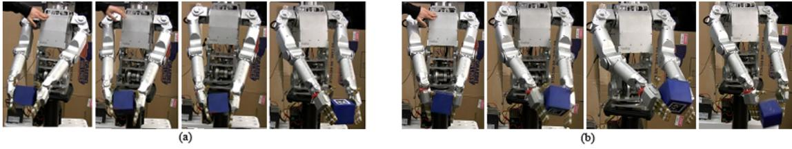
Fig. 4. Pushing the robot during a box-moving trajectory to demonstrate the response (a) without secondary augmentation and (b) using SIL.
