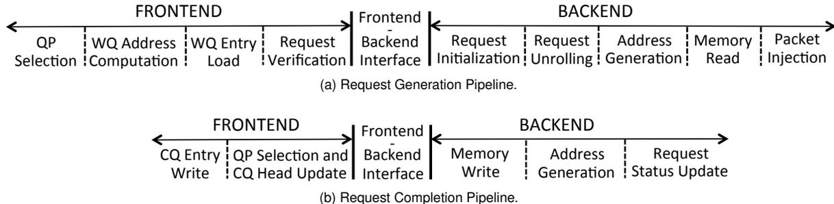
Figure 4: Scale-Out NUMA RGP and RCP pipelines.
