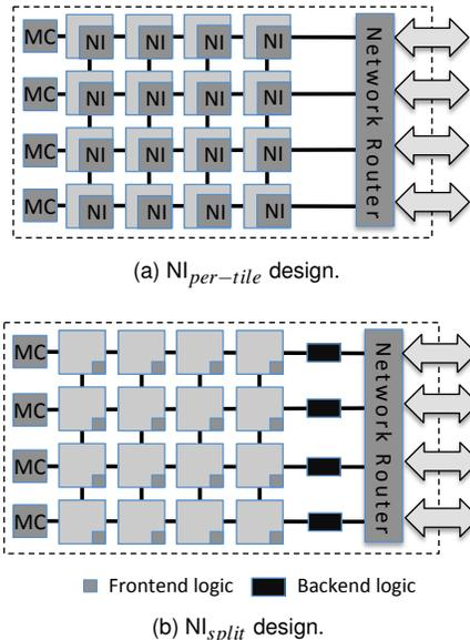
Figure 3: NI design space for manycore chips.
