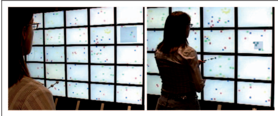
Figure 6. Using a wand to select at different scales based on distance from the display.
