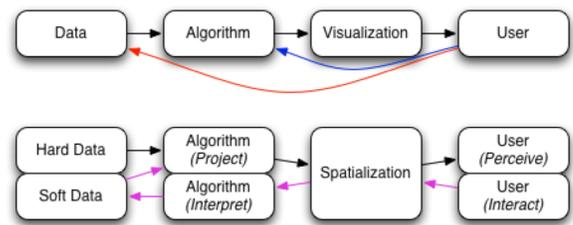
Figure 1. (top) The basic version of the “visualization pipeline”. Interaction is performed directly on the algorithm (blue arrow) or the data (red arrow). (bottom) Our modified version of the pipeline for semantic interaction, where the user interacts directly within the spatial metaphor (purple arrow). Analytic reasoning is interpreted and used.
