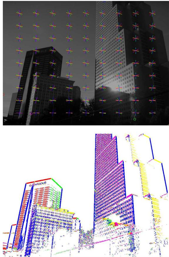
Figure 1: This scene contains two pairs of orthogonal, horizontal vanishing directions in addition to the vertical. In this paper, we introduce an EM-based method to recover vanishing directions (top) while simultaneously grouping edges (bottom). Each colored line segment in the top image is oriented along the vanishing direction of an identically colored edge group in the bottom image.
