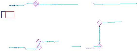
Fig. 1. The result of feature detection is shown together with the raw data. The raw laser range data is shown as black dots with the red/blue robot indicating the center of the range sensor. Incrementally fitted line segments are drawn as cyan lines, while diamonds represent corners detected as intersections of neighboring line segments.
