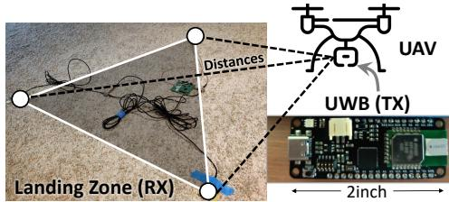
**Figure 4: Homecoming test LZ ranging with UAV**
