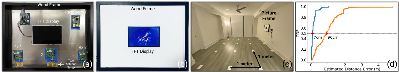
Figure 5: (a) The internal components include UWB devices, single-board computer, and TFT display. (b) External appearance with live visualization on the digital picture frame. (c) Evaluation space. (d) The blue line shows the absolute distance estimation error and the orange line shows the absolute location estimation error.
