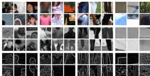
Figure 3: Example patches classified by humans as (left to right) head, torso, legs and background in (top to bottom) regular, grey-scale low resolution and normalized gradient images.
