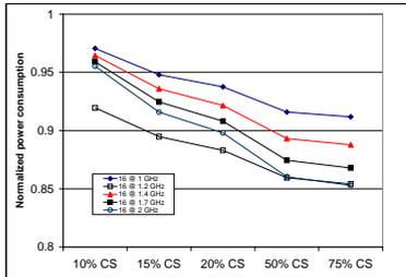
Fig. 5. Average power vs. different critical section length (normalized to the 16 thread matrix multiplication workload)
