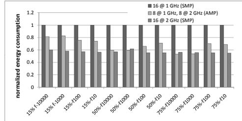
Fig. 7. Critical section frequency effects on performance and energy (left: execution time, right: energy consumption)
