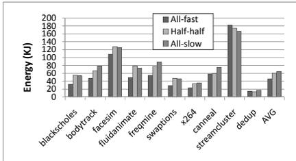
Fig. 3. Energy consumption behavior in three machine configurations (PARSEC)
