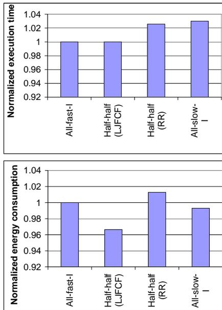
Fig. 10. The performance and energy consumption behavior of the ITK benchmark (top: execution time, bottom: energy)
