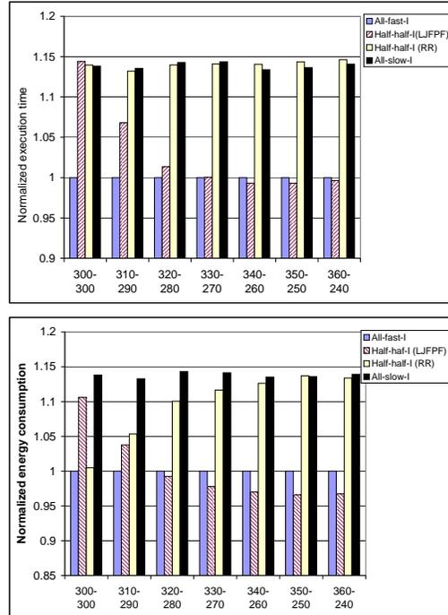
Fig. 9. The performance and energy consumption behavior in the matrix multiplication application with the LJFPF scheduling policy (top: execution time, bottom: energy consumption)
