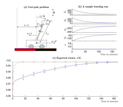
**Fig. 2.** Performance of Natural Actor-Critic in the Cart-Pole Balancing framework. (a) General setup of the cart-pole system. (b) A typical sample learning run of both the natural actor-critic (dashed line) and the true policy gradient (solid line). (c) The expected return of the policy over time. Curves are an average over 100 randomly picked policies as described in Section 4.1.
