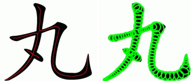
Fig. 7. A Chinese character with centerlines(left) and discrete pearls (right) computed by pearling in 37ms on an image with size 236x201.
