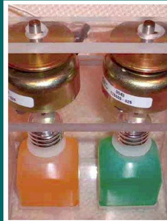
Solenoid-controlled scent bottles
