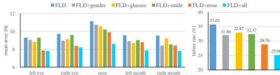
Fig. 1. Comparison of different model variants of TCDCN: the mean error over different landmarks, and the overall failure rate.
