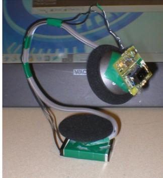
**Fig. 1.** The FreeDigiter device is equipped with a dual axis accelerometer, an infrared proximity sensor, and a Bluetooth radio for wireless communication. The entire device is worn like a pair of headphones with the sensors positioned over one of the ears.
