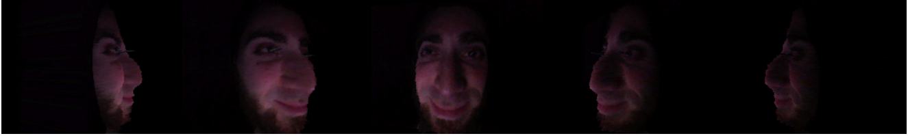
Figure 4. A recovered 3D model rotated through 180 degrees. The geometry of this model was recovered from the four images shown in Figure 1, while the texture was taken directly from only the first of the four images. Note that the virtual camera is placed close to the model to emphasize depth, leading to the extreme perspective distortion in these images.
