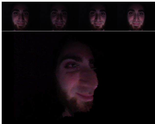
Figure 1. Using only the light from a computer screen to illuminate a face from multiple directions (top), we use photometric stereo techniques to recover a textured 3D surface (bottom) in real-time from live video. This technique is viable on any laptop or desktop computer with a screen and webcam.
