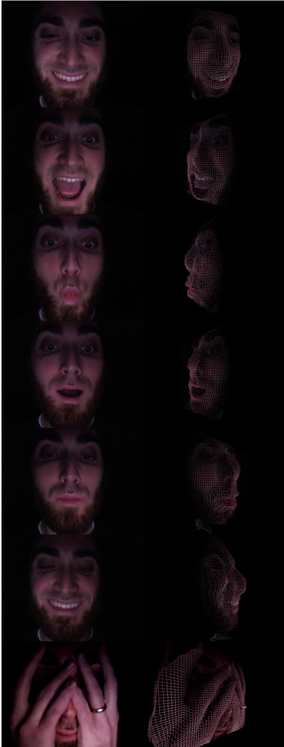
Figure 5. Example frames of live video (left) and corresponding real-time 3D reconstructions (right) displayed as textured wire-frame meshes.
