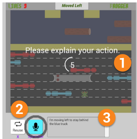
Figure 1: The rationale collection process. (1) Game pauses after each action. (2) Speech-to-text transcribes the rationale. (3) Participants can view and edit the transcribed rationales.
