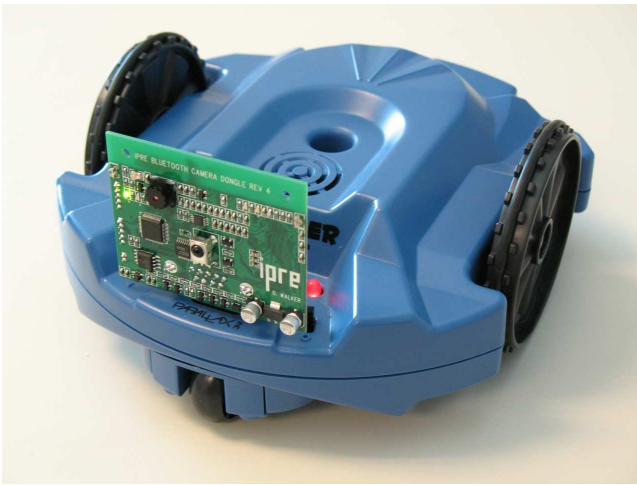
Figure 2: Parallax Scribbler with the Lancet Fluke upgrade board that provides Bluetooth, a camera, additional sensors, and LEDs.
