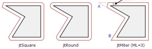
The angle at vertex 'A' is more acute than that at 'B' and, since a mitered offset would exceed the specified limit (3 x delta), its offsetting is 'squared'.
