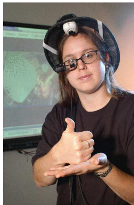
Figure 1. Prototype one-way translator (vision system only shown). The head-up display provides a 640x480 color interface for the signer.
