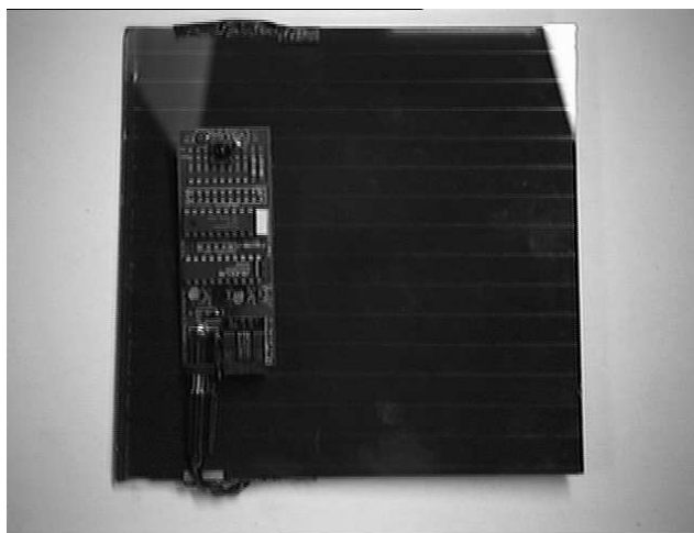
Figure 9: Environmentally-powered, microcontroller-based IR transponders.
