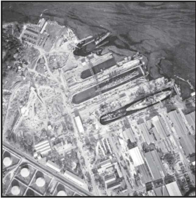
Figure 1. Aerial View of Pearl Harbor Drydock, 10 December 1941. Note the improvised antitorpedo barriers located near the drydock openings. USS Pennsylvania and the sunken destroyers Cassin and Downes are in the lower, No 1, drydock. The USS Helena occupies the middle drydock. The USS Shaw and the sunken drydock YFD-2 are on top. Numerous support shops and base facilities are located in the lower right corner. Also, note the black oil streaks on the harbor surface. 77
